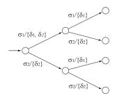
Fig. 1. Controlled discrete event system G of Example 1.
