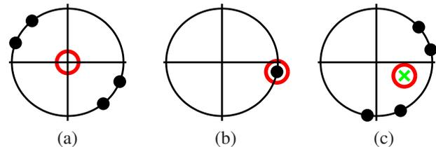
Fig. 1. Example headings are plotted on the unit circle as dark dots for (a) balanced, (b) aligned, and (c) reference matched group states with  $N = 4$ . The large red circle denotes the phase centroid. In (c), the reference vector is denoted by a green "x" located at  $[0.75, -0.25]$ . The work in this paper establishes stability to both balanced and reference matched sets.
