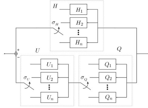
Fig. 2. Connection structure of a switched system  $H_\sigma - Q_\sigma V_\sigma$
