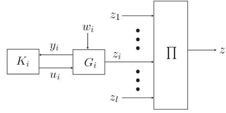
Fig. 4. Connection structure of a mixing system with  $l$  agents
