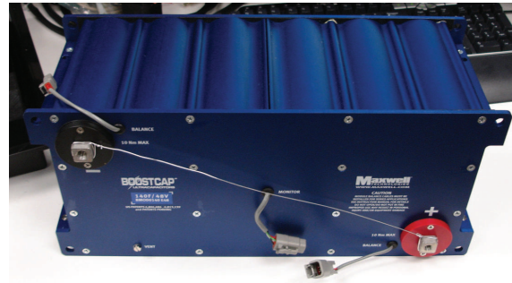
Fig. 1. The 48 volt BMOD0140 Maxwell ultracapacitor module with capacitance of 140F (Dimensions 41.6 \times 19 \times 16 cm, Mass \approx 13.6 kg). While the maximum total energy stored is a mere 161kJ, this energy can be released in just a few seconds generating considerable power boost to a vehicle. The maximum power for this product is 4800W per unit mass or almost 65kW instantaneous maximum power. Newer products listed on Maxwell website [4] have even higher power densities.
