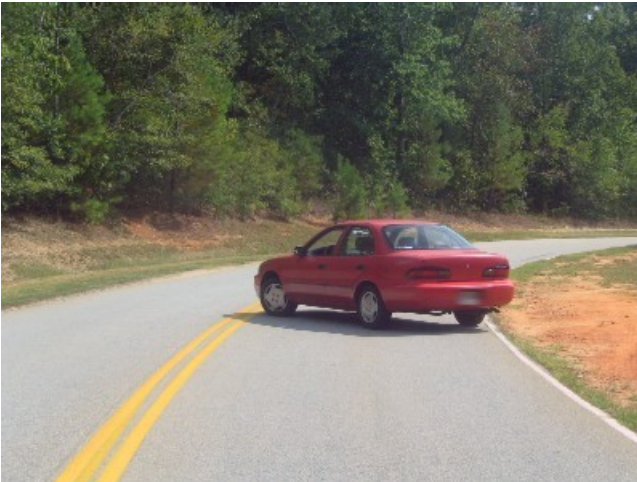
Figure 5: Vehicle less than one second after re-entry with large yaw angle and approaching roadway double solid line.
