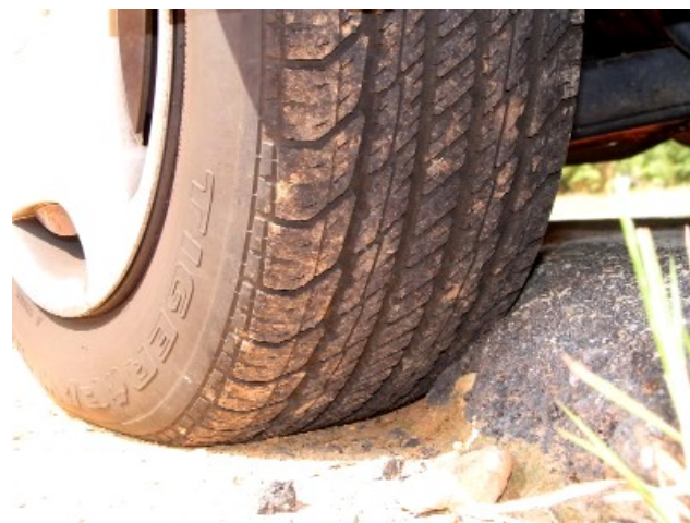
Figure 3: Front tire caught against the road shoulder prior to the vehicle’s return to the road surface.
