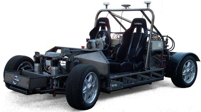
Fig. 1. Stanford’s P1 Steer-by-wire vehicle
