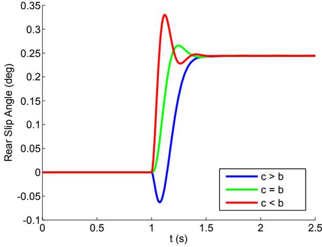
Fig. 6. Simulated  $\alpha_r$  response to a front step steer maneuver for various  $c$
