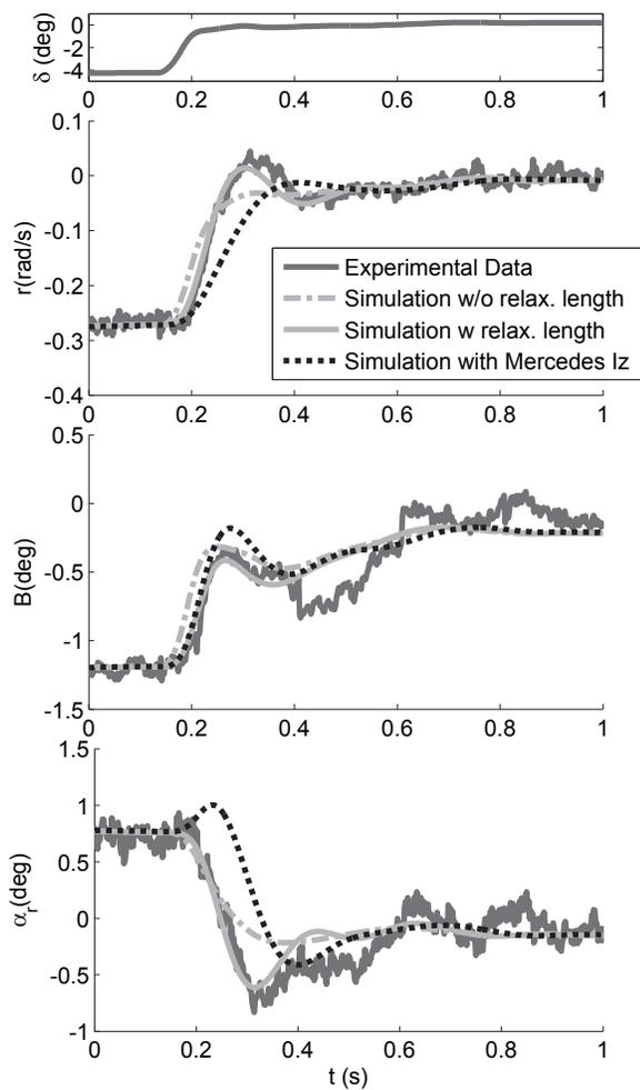
Fig. 8. Experimental response of PI to a fast ramp steer maneuver: a) steering input, b) yaw rate, c) sideslip, d) rear slip angle
