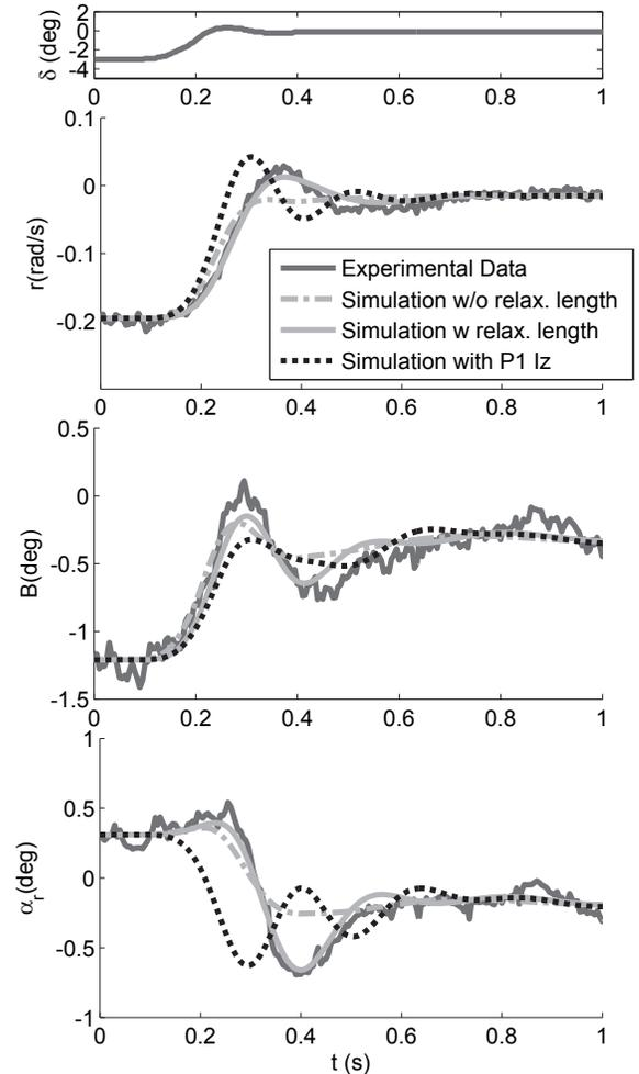
Fig. 7. Experimental response of the E320 to a fast ramp steer maneuver: a) steering input, b) yaw rate, c) sideslip, d) rear slip angle
