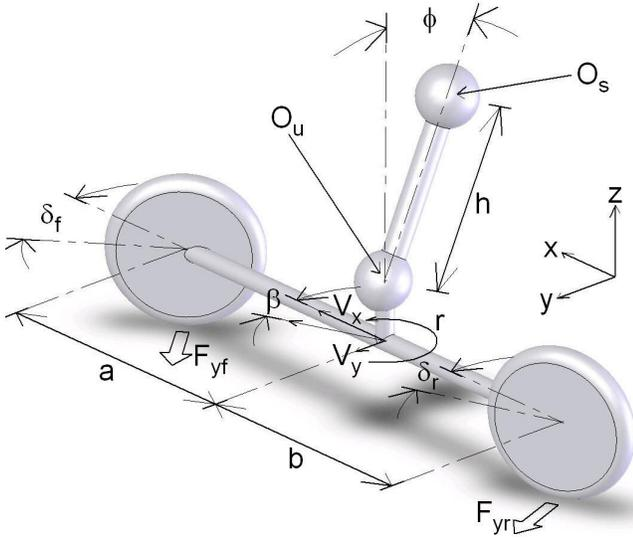
Fig. 2. Diagram of 3DOF Vehicle Model
