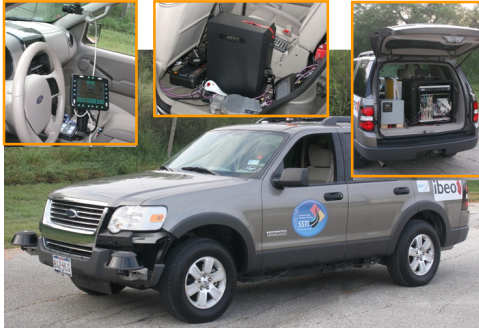
Fig. 5. The SSTI AGV vehicle and control/sensing systems.
