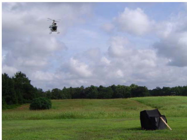
Fig. 13. Photograph of a vision-aided INS flight test, showing the helicopter hovering in the upper left and the black optical target in the lower right.
