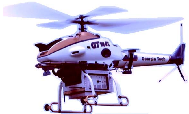
Fig. 3. GTMax Research UAV, utilized to test automated visual search approaches
