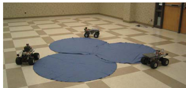
Fig. 6. Indoor experimental setup for perimeter detection.
