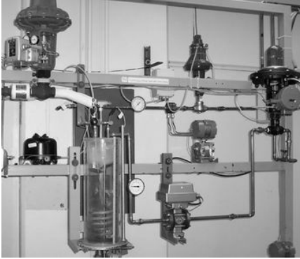
Fig. 2. Physical layout of the CSTHS system with the associated hardware
