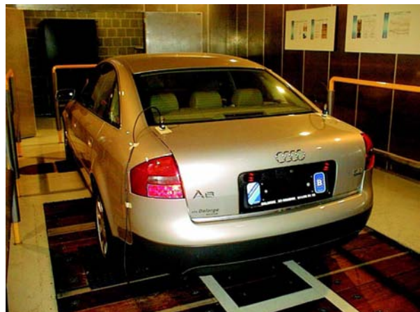
Fig. 3. Picture of the passenger test-car on the hydraulic shaker
