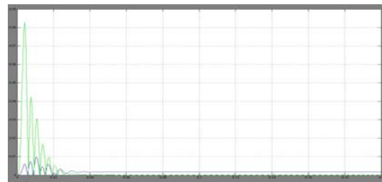
Fig. 10. Comparing two simulations with different values of on-state resistance (trend on standard deviation)
