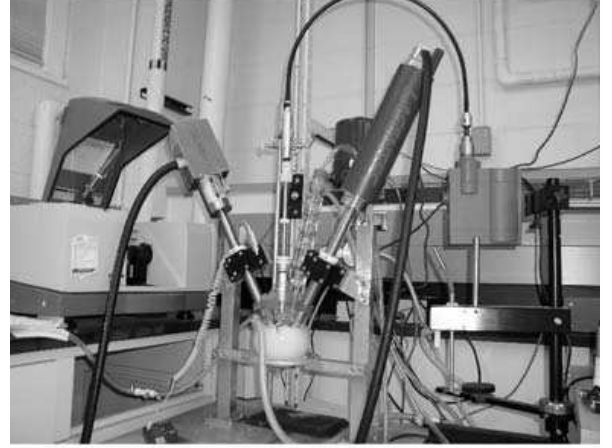
Fig. 1. Experimental set-up for suspension polymerization reactions. The in situ Lasentec FBRM (left) and Lasentec PVM (right) probes are used to measure the PSD.
