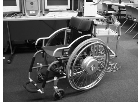
Fig. 1. Power-assisted Wheelchair as an Example of Power Assistance Tools (YAMAHA JW II)
