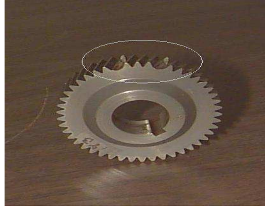
Fig. 4. Failure in the drive gear for test run 1
