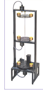
Fig. 7. The 3-disk Torsional Pendulum System [21].
