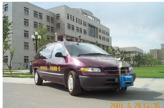
Figure 1. THMR-V: outdoor mobile robot of the fifth generation
