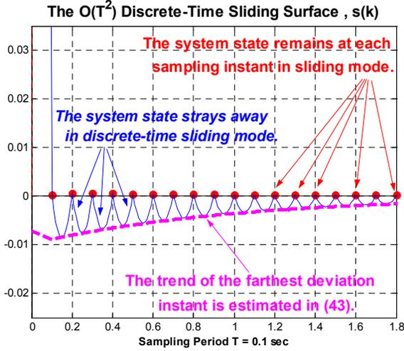
Fig. 1. An  $O(T^2)$  boundary layer in the discrete-time sliding mode
