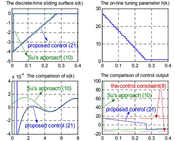
Fig. 3. The comparison with initial condition  $x_1(0)=-3, x_2(0)=-1$
