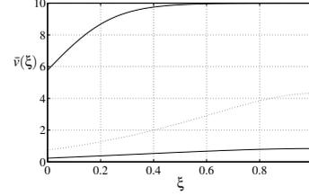
Fig. 6. Steady-state profiles for the adiabatic chemical tubular reactor with  $Pe = 3$ ,  $Da = 0.05$ ,  $\mu = 0.05$ , and  $b = 10$ .
