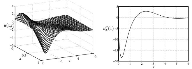
Fig. 7. Closed-loop response and the control effort for the chemical tubular reactor example.
