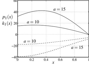
Fig. 2. Controller (dashed) and observer (solid) gains for the anti-collocated case.
