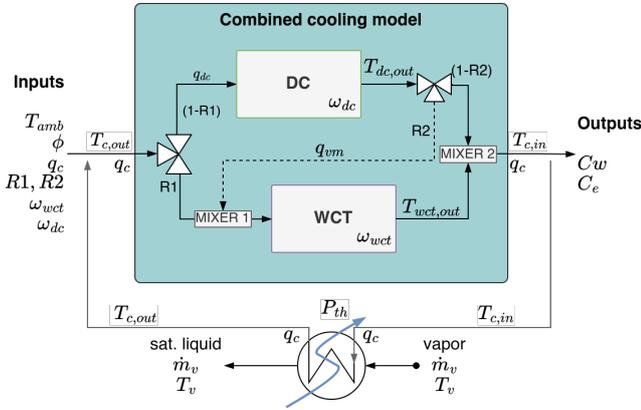
Fig. 3. Complete system model diagram
