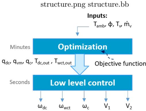
Fig. 2. Control structure
