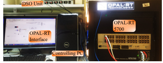
Fig. 5. OPAL-RT based HIL setup
