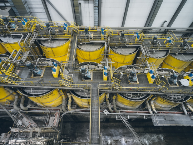
Fig. 1. Photo of a part of the flotation process in the Aitik concentrator, located near Gällivare, Sweden. Photo credit: Jonas Westling.
