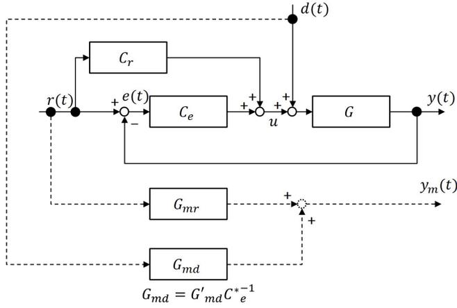
Fig. 1. Block diagram of a two-degree of freedom control system.
