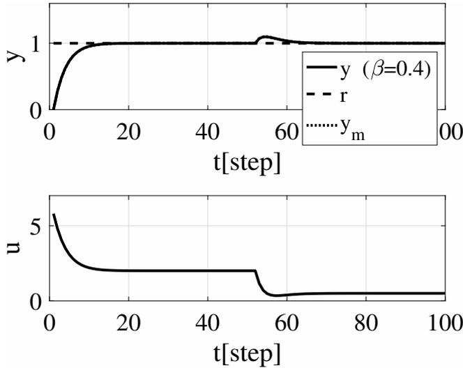
Fig. 4. Control results by using the proposed scheme ( $\beta = 0.4$ ).
