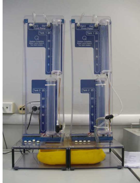
Fig. 1. Quadruple tank plant used in the remote laboratory. The plant is composed of two coupled tanks modules from Quanser ( www.quanser.com ).
