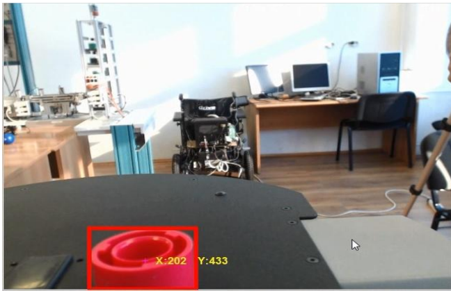
Fig. 8. Piece recovering using mobile visual servoing
