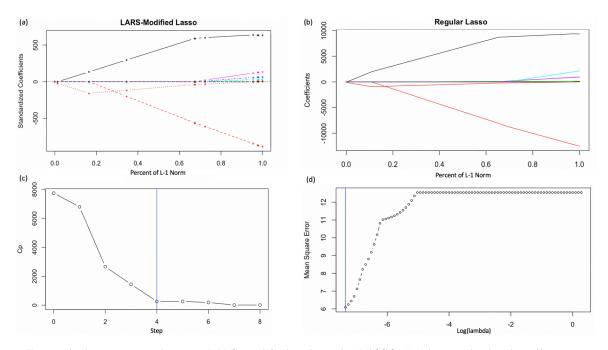
Figure 4. A comparison between LARS-modified and regular LASSO: (a) the standardized coefficient estimates using LARS-modified LASSO; (b)the coefficient estimates using regular LASSO; (c) the Cp value at each step for LARS-modified LASSO; and (d) the MSE at each lambda value in log scale. In (c) and (d), the blue lines indicate the steps of the best set of coefficients.
