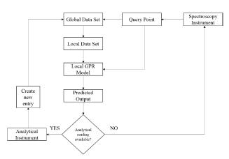
Figure 1: A flowchart for the proposed JITL-based Raman model.
