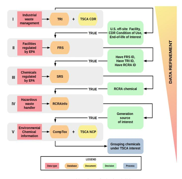
Figure 1. Data engineering and data refinement flowsheet for end-of-life scenario
