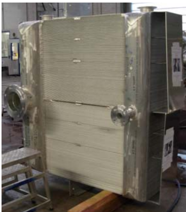
Figure 2: Photo taken during manufacturing of the first PFHE specimen
