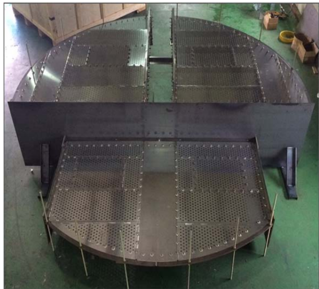
Figure 8a: Liquid Splitting Distributor in DWC column; Figure 8b: Dividing Wall Column Trays at Manufacturing Workshop
