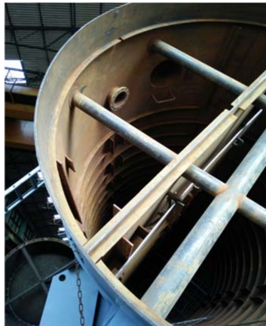
Figure 2a: Proprietary DWC Process Scheme; Figure 2b: Inside View of a Top Dividing Wall Column
