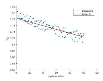
Fig. 5.  $V_{0+}$  vs. Cycle Number - with linear fit
