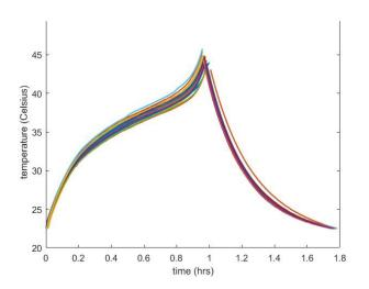
Fig. 7. Temperature (normalized) vs. Time for CCD and  $\operatorname{OCV}$
