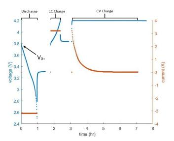
Fig. 2. Discharge/Charge Current and Voltage Profile
