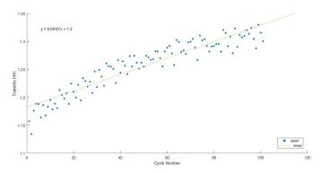
Fig. 6. Capacity vs. Cycle Number for constant voltage charge
