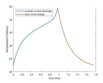
Fig. 8. Average Temperature (normalized) vs. Time for CCD and OCV
