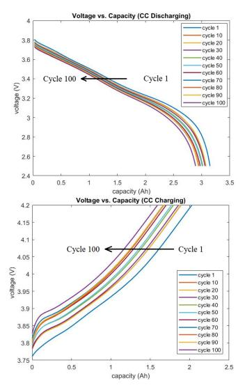
Fig. 3. Voltage vs. Capacity curves for a) constant current discharge and b) constant current charge
