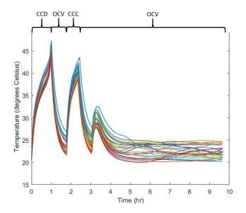
Fig. 4. Battery Temperature vs. Cycles
