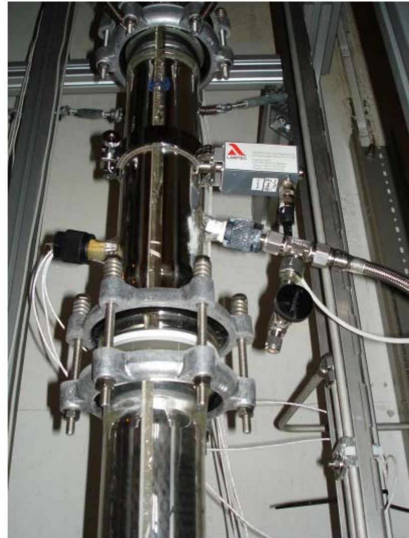
Figure 7.2: Side-stream product draw. Swinging funnel inside column section directs the liquid to the product line or as reflux.
