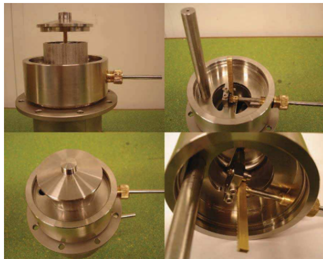
Figure 3.3: Picture of dismantled vapor split valve, [DWIVEDI 2013]
