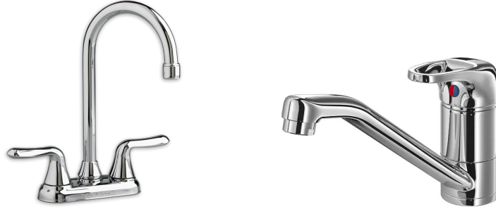
(a) Traditional design with two separate handles ( u_1 = F_1 , u_2 = F_2 ) (b) Modern one-handle design where decoupling is achieved by the physical design ( v_1 = F_1 + F_2 and v_r = \frac{F_1}{F_2} ).
