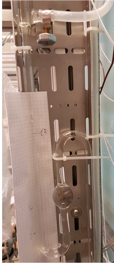
Figure 2.6: Picture of liquid seal positioned on product stream. It ensures that the vapor is not leaking through product stream.
