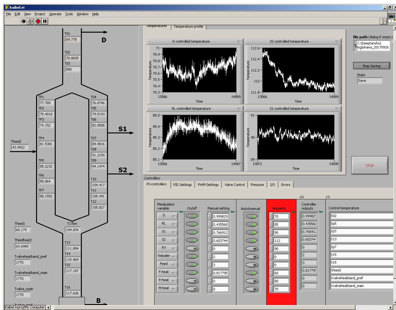
Figure 4.1: User interface in LabVIEW used for operation of Kaibel column.
