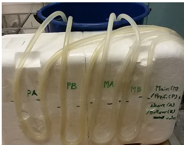
Figure 5.2: Liquid seals for pressure measurement above (A) and below (B) vapour split valves in prefractionator (P) and main column (M)
