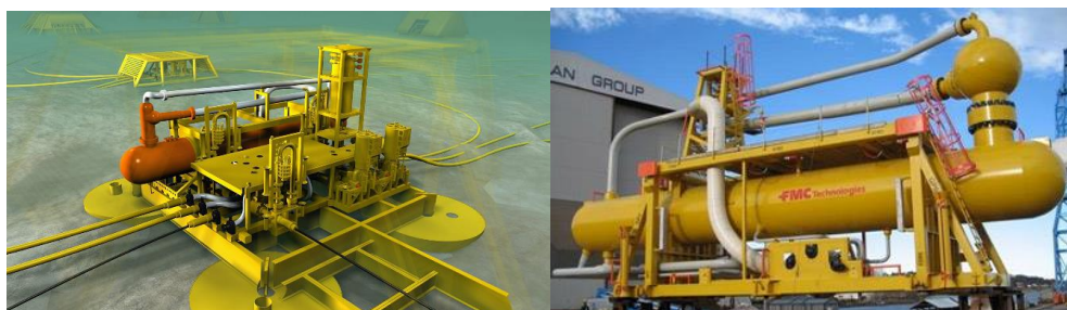
Figure 3: Tordis gravity separator , on the left graphical representation of Tordis on sea bed. On the right, actual picture of Tordis gravity separator taken in June 2007. The separator ensures that residual oil droplets are discharged into separate subsea wells instead of the sea.
