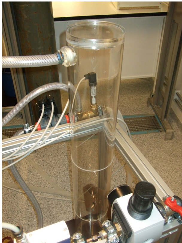
Figure 3.3: The air buffer tank.
