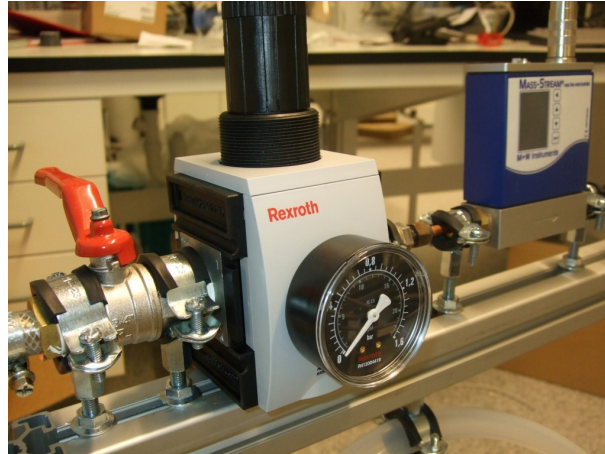
Figure 3.10: Manual pressure regulator from Rexroth.
