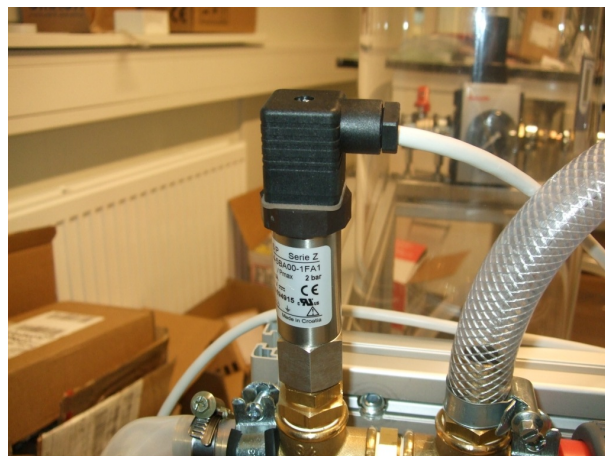
Figure 3.9: Pressure transmitters from Siemens.
