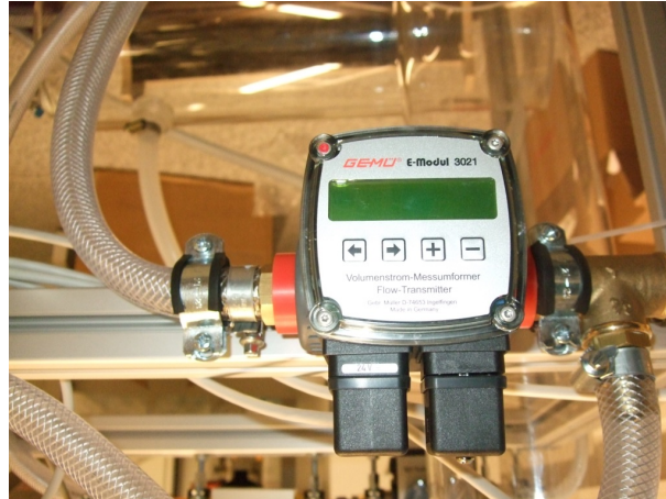
Figure 3.8: Liquid flow meter
