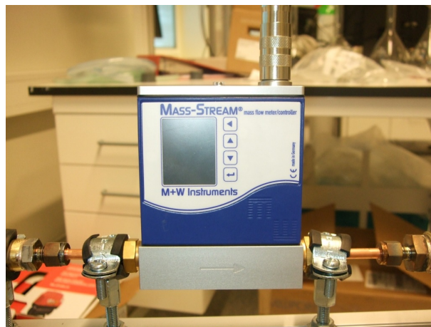
Figure 3.7: Air flow meter from M+W Instruments.
