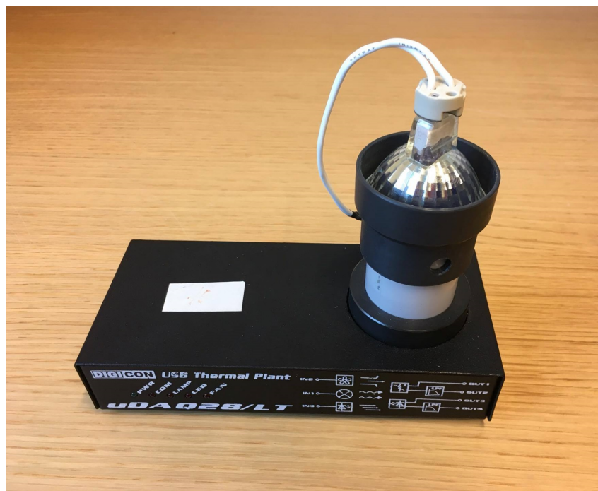
Figure 4.38: The thermal/optical plant uDAQ28/LT.
