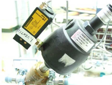
Figure 3.13: The choke valve used before the separator
