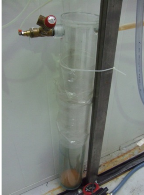
Figure 3.5: The air buffer tank.
