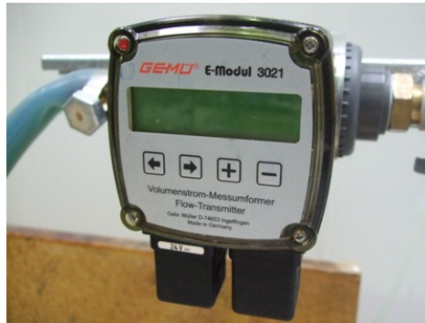
Figure 3.10: Liquid flow meter
