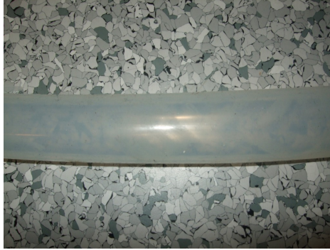
Figure 3.8: Transparent rubber tube, 20 mm inner diameter
