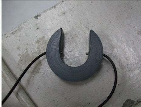
Figure 3.14: Fiber optic slug sensor by Omron.
