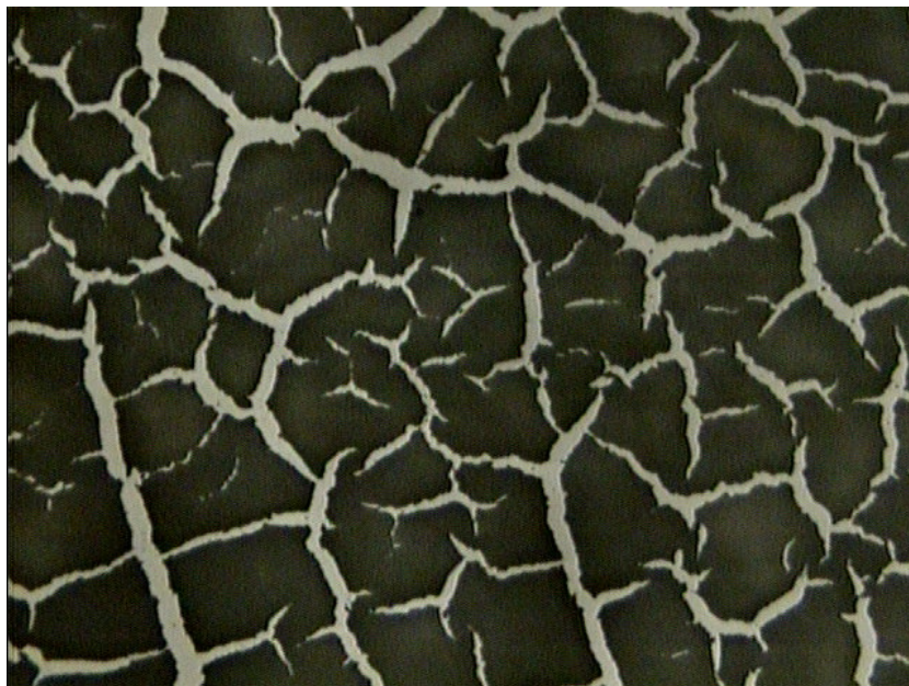
Figure 5.33. Dip coating micrograph of BESO 0.2 M (Sample eIII), 10x (glass slide).
