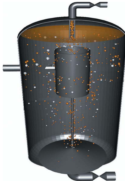
Figure 4.4. Principle of the Epcon compact flotation unit [32].
