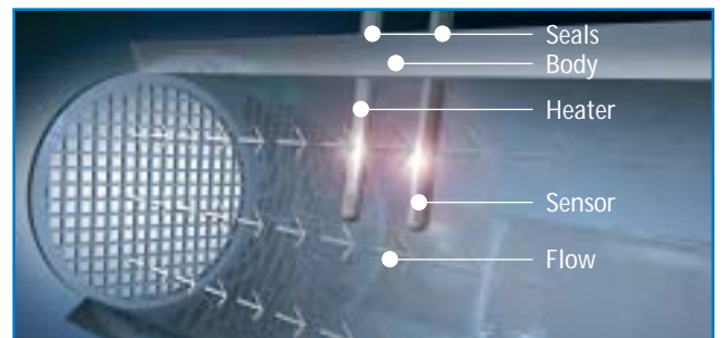
Basic structure of the MASS-STREAM®-flow sensor
