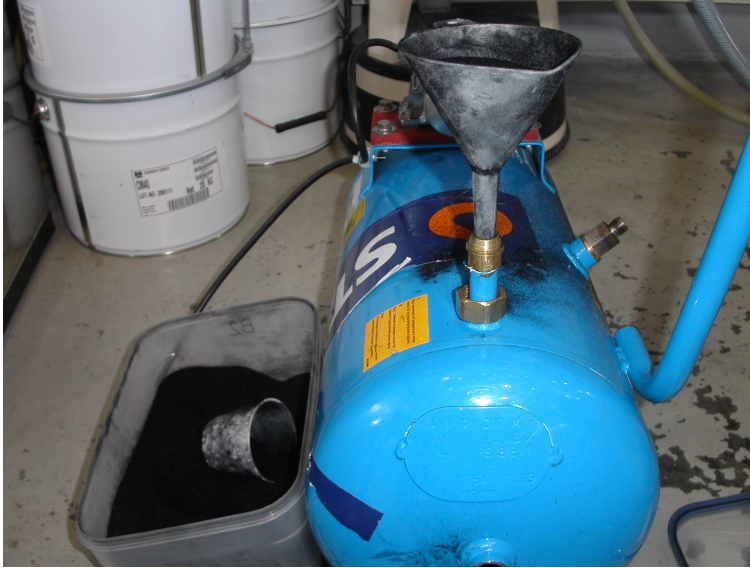
Figure 4.4.1: Particle/ fiber tank with polyamide.
