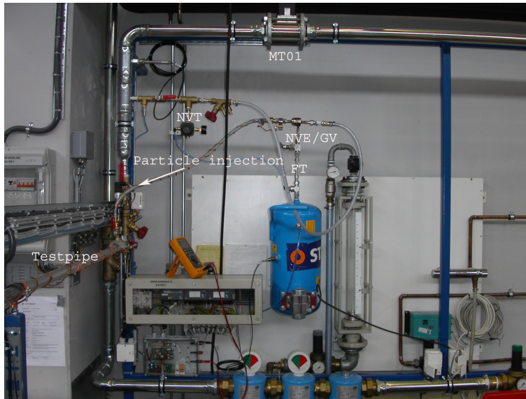
Figure 3.1.2: The injection system.
