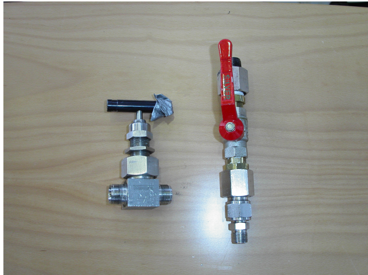
Figure 3.3.1: Needle valve (NVE) and global valve (GV) in injection system.
