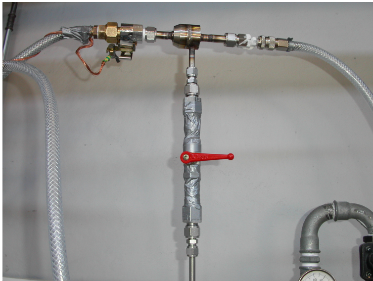
Figure 3.3.3: Jet mixer in injection system.
