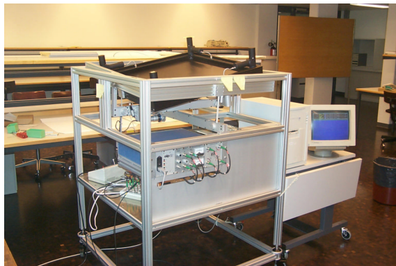
Figure E.2: Photo of “Ball & Plate” system.
