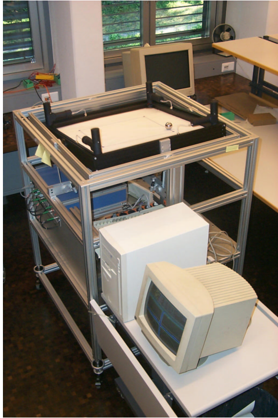
Figure E.3: Photo of “Ball & Plate” system.
