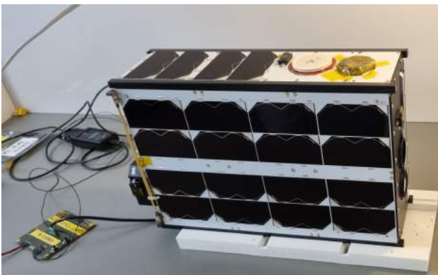
Fig. 2: An image of the 6U CubeSat going to space during final system check at the CubeSat vendors facilities.
