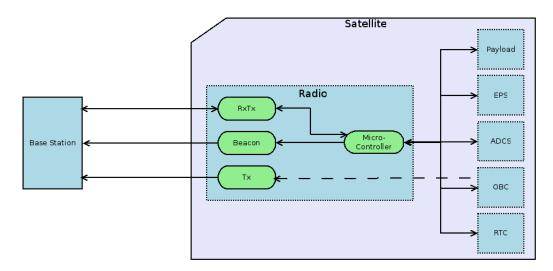
Figure 1. Schematic overview of the communication structure
