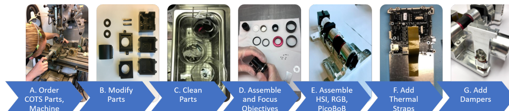
Figure 9. Simplified assembly sequence for the HYPSON-1 payload at NTNU.
