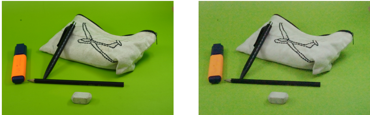
Figure 2.9: The impact of ISO sensitivity on the image quality. Pictures made with ISO value set to (a) 100 and (b) 65535 with equivalent exposures and same aperture sizes.
