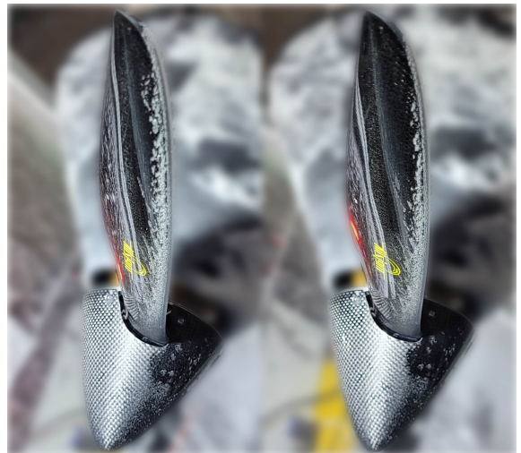
Figure 11: 40 s ice shape before (left) and after (right) the multistep experiment.
