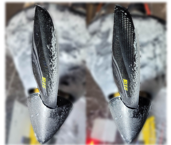
Figure 12: 60 s ice shape before (left) and after (right) the multistep experiment.
